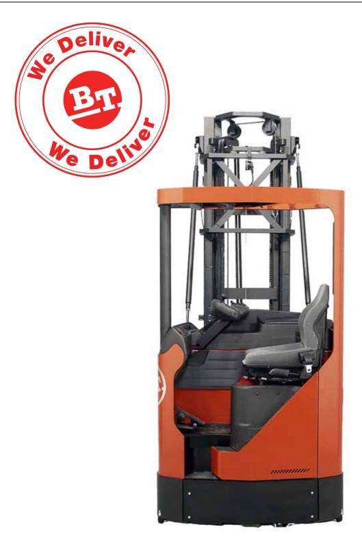
The Veflex is equipped with everything needed for heavy duty and high performance very narrow aisle handling. As a special version, the Veflex VRE125 is available with a duplex mast, allowing a great forward view. Furthermore, a redesign of the mast fitting has resulted in an improved visibility over the forks at low level.
