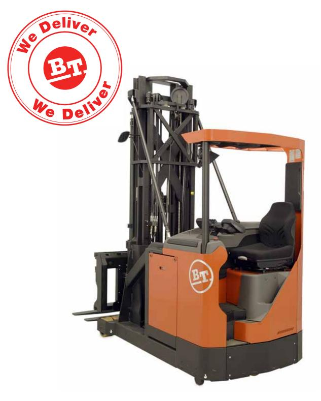
The Veflex is a very narrow aisle truck, based on the successful technology of the Reflex reach truck. It is equipped with everything needed for heavy duty and high performance very narrow aisle handling.
