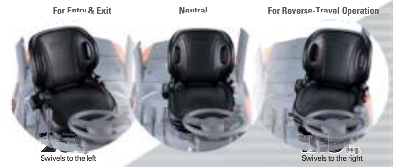
Swivel Seat OPT The seat swivels 17.5 degrees to the right, enabling the operator to maintain a comfortable posture when reversing. The seat also swivels 20 degrees to the left, makes getting off even easier.
