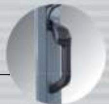
Rear-pillar Assist Grip OPT This assist grip with horn button supports the driving position and offers easy horn operation while traveling in reverse.
