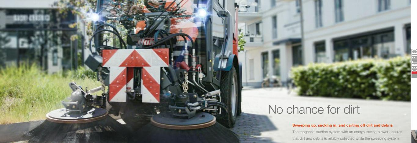
The tangential suction system with an energy-saving blower ensures that dirt and debris is reliably collected while the sweeping system goes easy on pavements and joints, and our efficient separation system provides maximum filling of the universal hopper – for extended emptying intervals and a higher payload.
