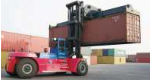
Stacking heavy containers (24-45 tons) up to 5 high.
