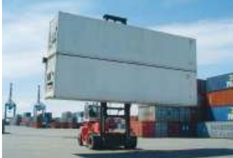
Double up. Equipped with a special double-stacking attachment, this truck empties containers with unbeatable speed.
