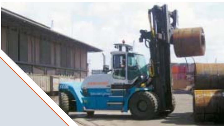
Handling larger coils and slabs requires bigger trucks (10-60 tons).
