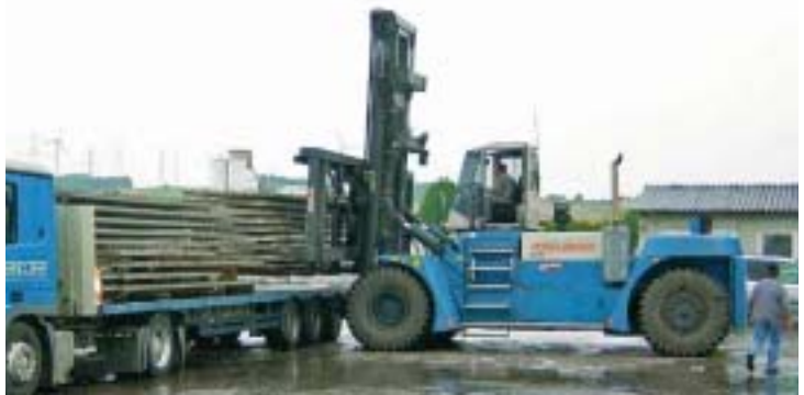
Handling heavy concrete elements requires a wide carriage and side cabin (16-42 tons).
