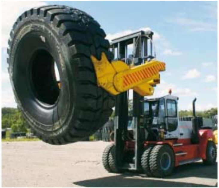
Changing tires on giant mine trucks requires precision (15-25 tons).
