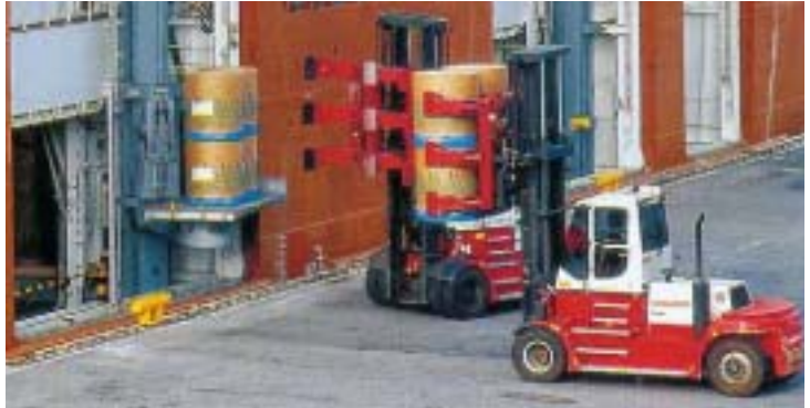
Secure grip of paper rolls. Handling 2, 4 or 6 rolls in the attachment (12-16 tons).
