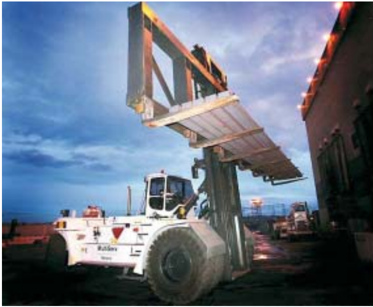
Raw power for heavy raw materials. Lifting steel slabs and coils requires large trucks – up to 60 tons.
