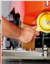
Overview at a glance: Wear indicator for brushes and pads. A comfortable discharge system enables fast and easy changing of the brushes – without the need for tools.
