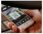
Service via code scanning: The QR code below the steering wheel allows access to all relevant machine data and other details – even transmitting service requests directly there and then.
